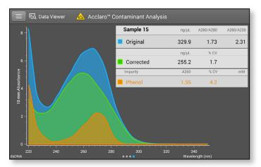
dsDNA sample contaminated with phenol. The absorbance contribution from the phenol (orange) is subtracted from the original result (blue) to obtain the corrected dsDNA concentration (green).
